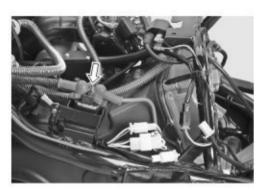
Connect terminals ① and ② to 12V voltage, inspect conductivity between connectors, positive and negative terminals. Starting relay is inspected to be conductive if it is free from damage.
