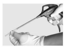
Disassemble fuel filter and inspect paper filter strainer. Replace it if it is obviously dirty.
