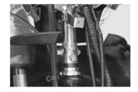
• Remove steering stem lock screw ① with universal clamp wrench:
