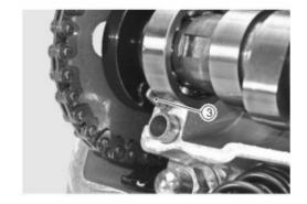
Mount cam chain tensioner 4 with bolt 5;
