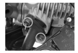
• Remove muffler mounting bolt and air exhaust pipe subassembly,
