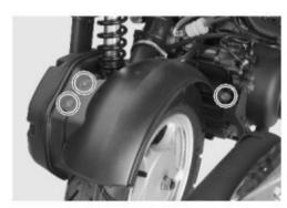
• Remove mounting screw, loosen carburetor clip and remove air cleaner case;
