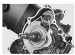
Remove crankshaft with special tool;
