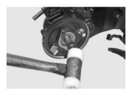
Remove nut, bolt, rear brake cam swing arm, brake lining wear indicator and brake cam;
