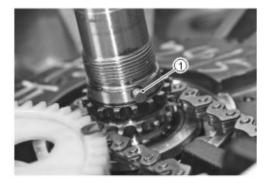
Tighten oil pump drive gear nut to specified torque by means of connecting rod.
