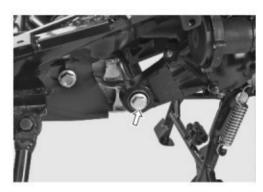
Loosen clip ① and disconnect air cleaner hose from carburetor,
