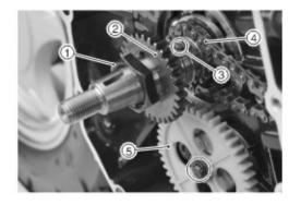
Remove oil pump screw and oil pump;
