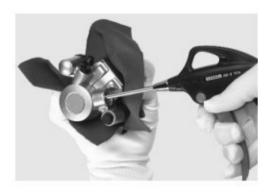
Remove the dust seal (5) and piston seal (6);
