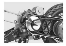
Remove clutch outer disc nut with special tools;
