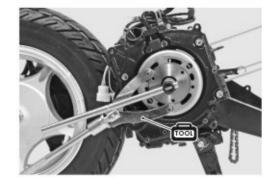
Remove magneto motor rotor with special tools;
