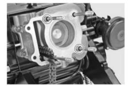
Mount cylinder head on cylinder with cylinder head nut and gasket fixed at correct positions.
