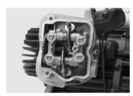
• Remove bolt and cam chain tightener ③;
