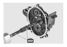
Remove drive shaft right bearing ① and idler shaft right bearing
