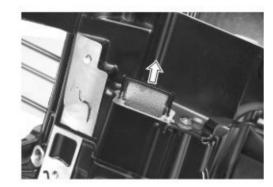
• Remove screw and engine oil filter cap;
