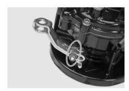
Mount rear drive shaft ① in crankcase by gently knocking drive shaft;
