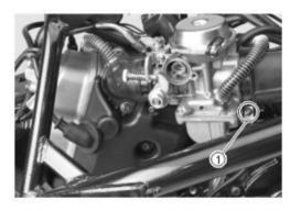
Remove carburetor dust board;
