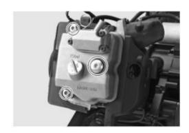
After removing spring carrier arm screw ①, remove mounting bolt and cam chain tightening adjuster;
