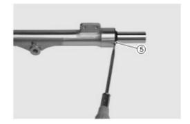
Remove buffer rod bolt with special tool;
