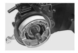
• Remove real wheel axle by knocking it with a plastic hammer;
