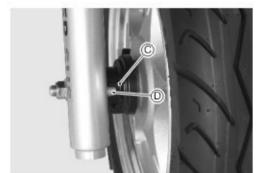
Connect speedometer flexible shaft ①.
