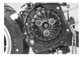
Remove magneto rotor nut with special tools;
