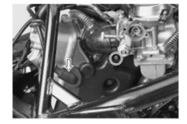
Remove mounting bolt and rear shock absorber;
