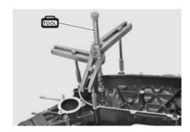
• Remove engine driven gear ⑥ by removing retaining ring ④ and washer 6;
