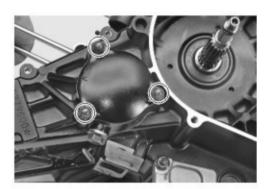
• Remove engine oil filter strainer and O-ring;
