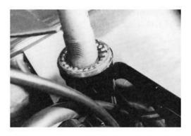
• Push out steering bearing upper race (5) and lower race (6);
