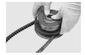
Mount clutch centrifugal shoe block together with sliding driven pulley subassembly and drive belt;
