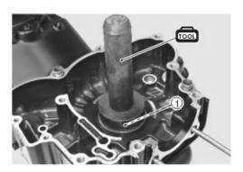
Mount crankshaft left oil seal ② with special tool;
