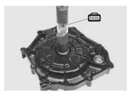
· Mount crankcase right cover oil seal with special tool;
