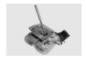
Trim cylinder head valve collar hole with reamer ① and reamer holder (2):
