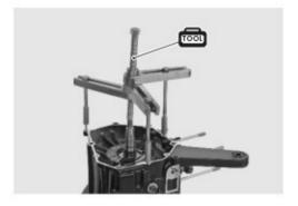
• Remove engine starting idle wheel ①, bush ② and axis pin ③;
