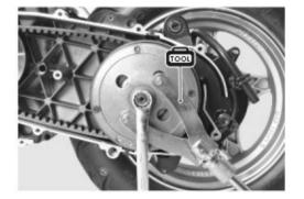
• Remove clutch centrifugal block, sliding driven pulley and fixed pulley subassembly;
